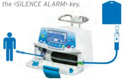
1. Align the tubing set horizontally along the tube guides so that the green connector is positioned to the right (green) and the blue clamp is positioned in front of the clamp guide (blue).
