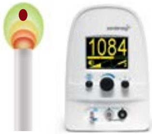
Pivot the probe around the hotspot to maximise the signal
